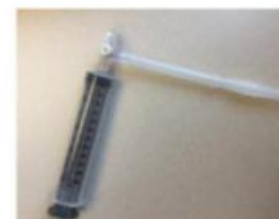
Photo of Luer-lock and tubing that connects to CT just above.
